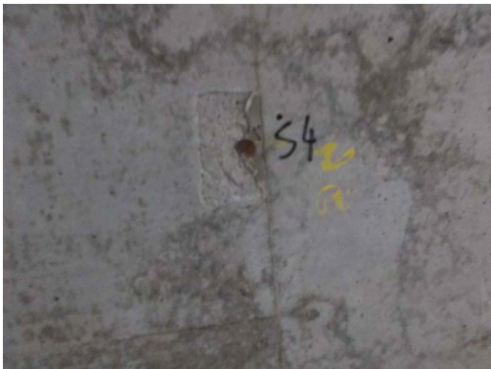
Photo C (up) Photo of the thermocouple on the exposed side of the slab - Section S3. Photo D (down) Photo of the thermocouple on the exposed side of the slab - Section S4.
